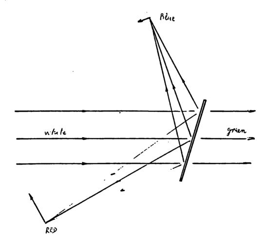
A single HOE can be used to replace lenses prisms and spectral filters.
